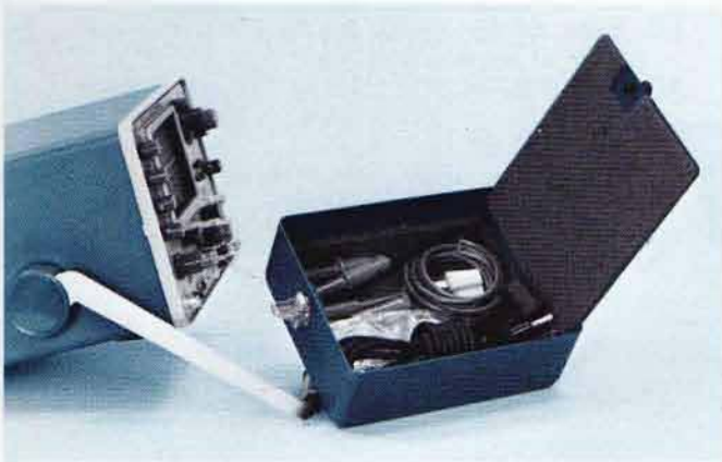
Panel dust cover provides storage for standard accessories.
