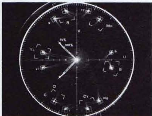
Fig. 1A—Vector PAL presentation of PAL color bar signal.
